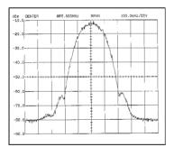
In digital mode the user can introduce defined errors to the modulation as skew, gain imbalance and carrier leakage, and so aid investigation of design limitations.
